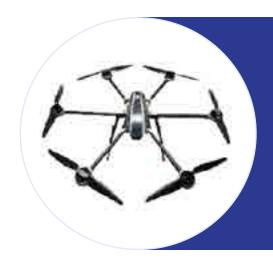
Heavy load foldable six-rotor UVA is long time for sailing and big load. Folded structure, mooring module, it can monitor the designated point in the sky for more than 10 hours. Maximum load: 15kg. It can carry some modules that have varied functions. It can meet the application of different practice.
