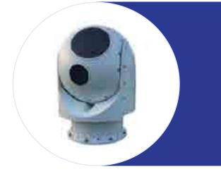
AresX<sup>™</sup> heavy-duty shipborne system using advanced ball-type dualframe, two-axis gyro stability and computer control system. While maintaining high-precision image, it ensures that the full enclosure and wind resistance of the optoelectronic devices. It suits the harsh environment at sea for all-weather target monitoring and search.
