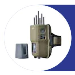
It is a six band handheld jammer. Easy operation and user friendly. It can be used for all the worldwide network frequency system. It is with an internal battery can support 1 hour lasting work.
